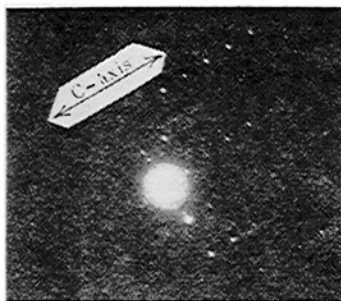
Fig. 4. N-pattern of the new hydrate (electron beam \perp c-axis).
